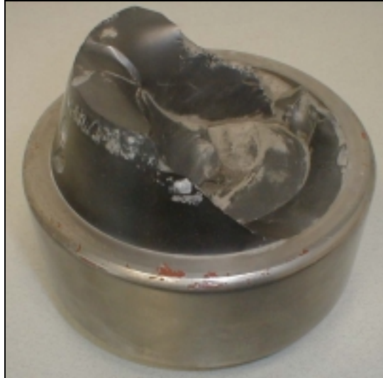
Typical Failure of Flash Letdown Plug Photo Courtesy of Caldera Engineering
